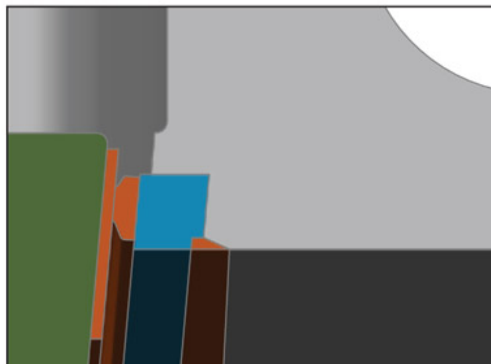
Welded Seat Ring With Stellite 6
